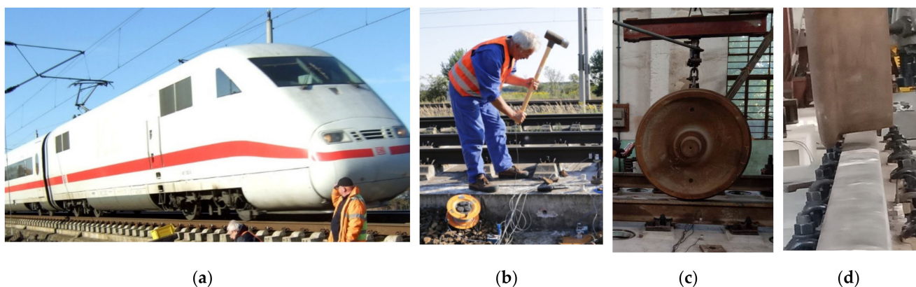
Figure 1. Experimental methods for identifying track properties and damage: (a) train passage at Site G; (b) hammer impacts at Site W; (c,d) wheelset drop tests at Site T.
