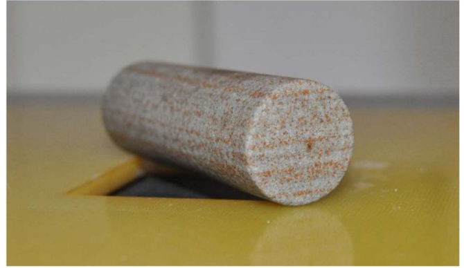
Figure 4. Berea sandstone sample on the SiS NMR sensor. The photograph was arranged to make the stratification of the rock visible. During the regular measurements of this study, the samples were covered in plastic foil to prevent evaporation during the NMR experiments.
