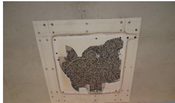
Figure 13 Photograph of the mobile furnace test specimen immediately after the fire test (mobile furnace test)
