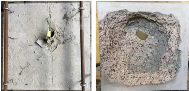
Figure 7. The result of an extensive explosion that took place while testing the loaded concrete slab in biaxial compression.
