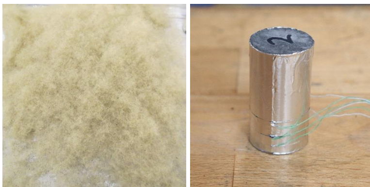
Figure 1 (a) Cleaned and untangled RTPF (b) Concrete specimen in aluminium foil.
