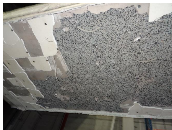
Figure 11 Photograph taken after the specimen was taken out of the furnace (large scale test)
