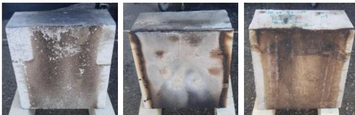
Figure 7 Specimens after fire exposure: Thin board mortar (left); Mortar board (middle), Concrete (right)
