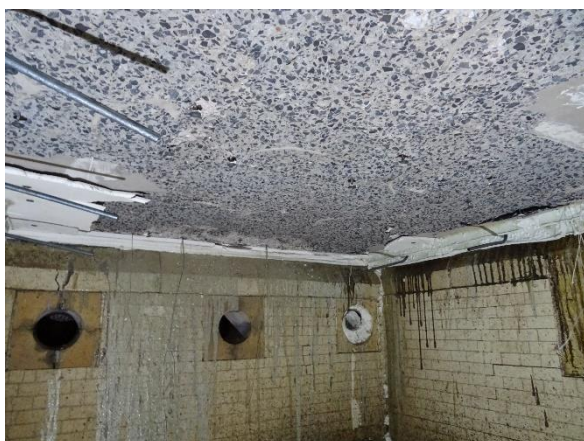
Figure 10 Photograph taken in the furnace 1 day after the fire test (large scale test)
