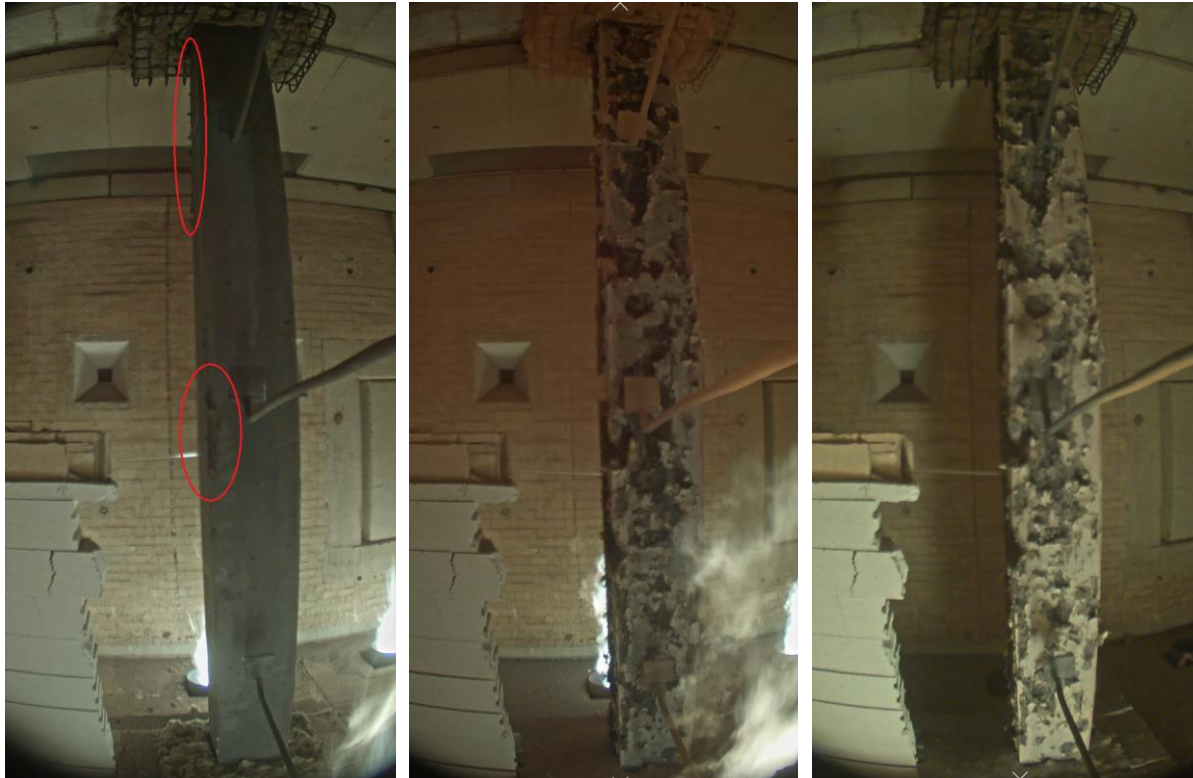
Figure 4 UHPC column during thermal exposure according to temperature-time curve T2 after 19 (left), 34 (middle) and 120 (right) minutes
