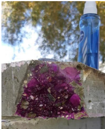
Figure 8 Carbonatisation depth example
