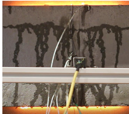
Figure 12 Longitudinal cracks developing at the unexposed face when exposed to simulated HCM fire curve
