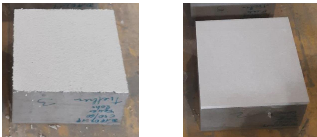
Figure 4 Lime-based thin bed mortar (left); Plasterboard (right)
