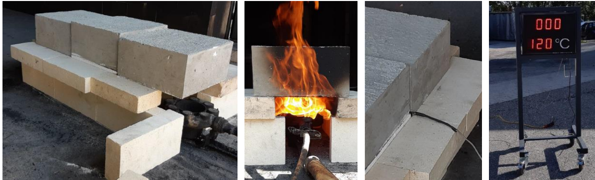
Figure 5 Experimental configuration (1); Burning specimen (2); Temperature probe position (3); Digital scoreboard (4)
