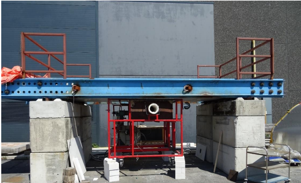
Figure 5 Experimental set-up for mobile Furnace test
