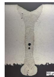
Fig. 3. Bright-field image corresponding to a full-penetration bead-on-plate. The base material is an AM-45° sample. The laser beam was directed to the smooth surface (up-skin)
