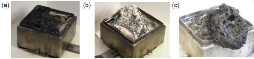
Fig 3.2.4.2 Fire residues of (a) PC/BDP, (b) PC/SiR and (c) PC/SiR/BDP obtained from cone calorimeter under 50 \text{ kW m}^{-2}
