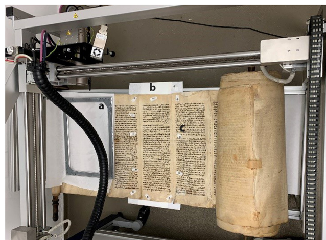
Fig. 1. Rhineland 1217 mounted on the stage, with (a) a weight used to flatten the unrolled part of the scroll; (b) the magnetic frame wrapped in acid-free paper; and (c) neodymium magnets, on acid-free paper washers, used for temporary noninvasive flattening of relevant portions of the scroll. The scroll is mounted upside down to give better access to the final columns.
