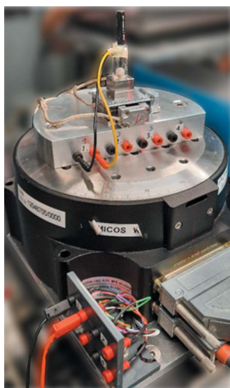
Figure 4 A slip ring offering eight channels (each with currents of up to 1 A) to facilitate cable management during rotation of the sample stage.
