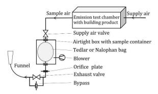
Fig. 3 - Adapter setup and positioning.
