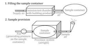
**Fig. 1 -** Sample provision setup using sample containers according to ISO 16000-28 (two sub-steps).
