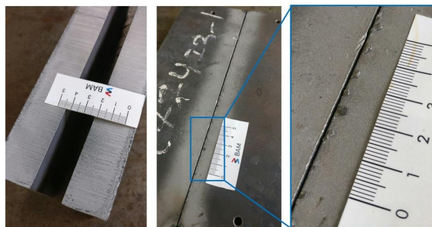
Figure 1. A 30 mm thick weld specimen EH36 with plasma cut edges.
