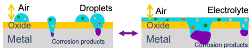
FIGURE 10 Schematic representation of the essential subcomponents of atmospheric corrosion. [Color figure can be viewed at wileyonlinelibrary.com ]
