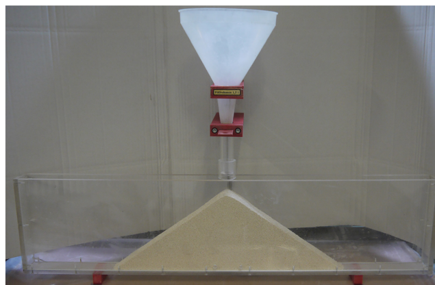
FIGURE 6 ‘Plate method’ (plexiglass): Test set-up—Eskal 0.5–1.0
