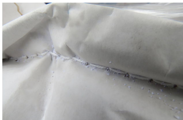
FIGURE 2 Release of a corrosive solid (UN No. 3262) from the seam of a 5M2 paper bag (Police North Rhine-Westphalia Münster)
