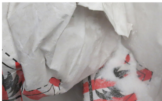
FIGURE 1 Release of a flammable solid (UN No. 1328) from the closure of a 5M2 paper bag (Police North Rhine-Westphalia Münster)
