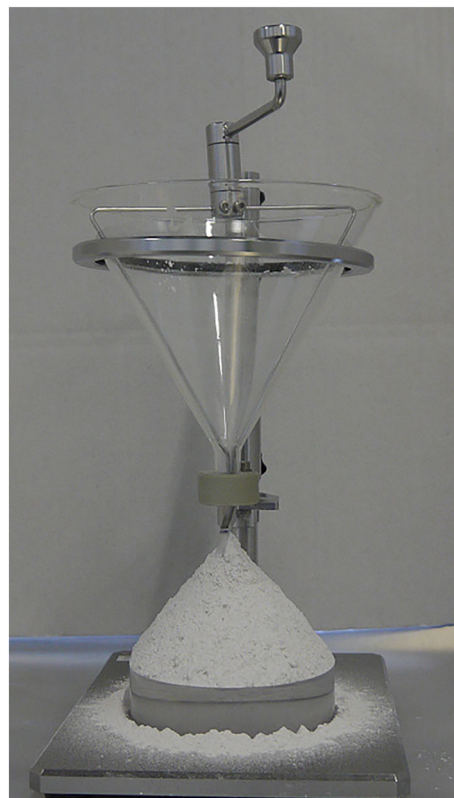
FIGURE 3 Method according to ISO 4324: Test set-up—Arizona dust A4 coarse
