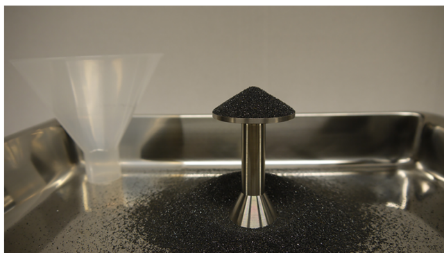
FIGURE 5 ‘Funnel test’: Test set-up—chrome ore sand
