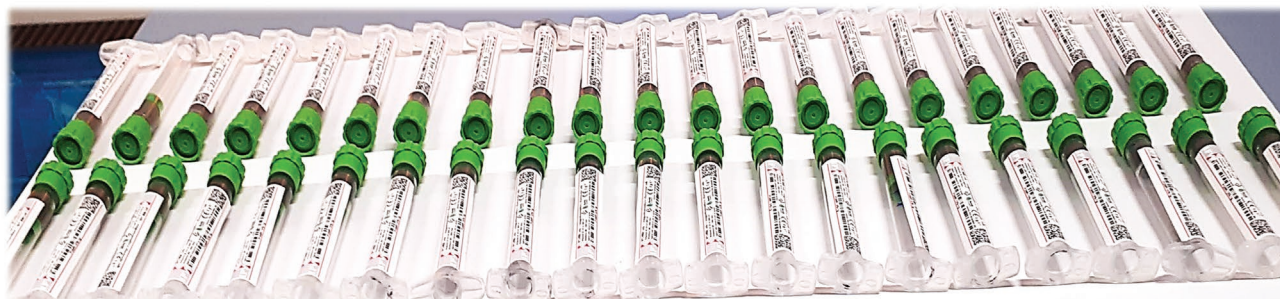
Figure 4. GMR ink preparation: a) Polyepichlorhydrin (PECH) polymer is mixed with ethyl acetate and stirred for 12 h at 50 °C to give final product and further loaded inside the cartridge and labeled as a binder cartridge. b) Magnetosensitive ink formulation: cartridge is loaded with weighed i) GMR powder and ii) PECH binder. iii) Dual luer-lock binds both cartridges for mixing and homogenization of the ink making the magnetosensitive (GMR) ink ready to use for printing. c) Represents the batch of 42 cartridges prepared from one single 100 m long magnetosensitive roll.
