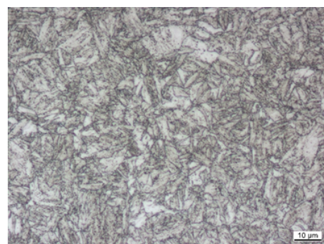
Figure 5. S690QL microstructure (T-L plane).
