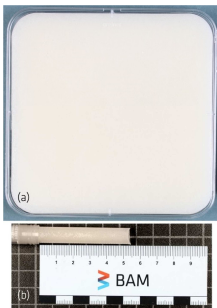
Figure 2. Gel-bound indicator (a) pad shaped (b) bar-shaped (stick).
