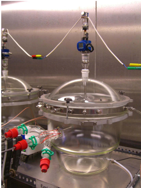
Figure 2.14: 24 l Emission test chamber
