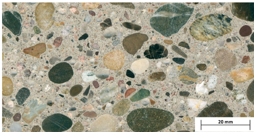
Figure 1. Typical concrete meso/microstructure: aggregate made of multicomponent river gravel, solidified by a cementitious binding matrix (mineral phases of micro- and nano-size, composed of relicts of the original binder and filler components and their multiphase reaction products resulting from their reaction with water).
