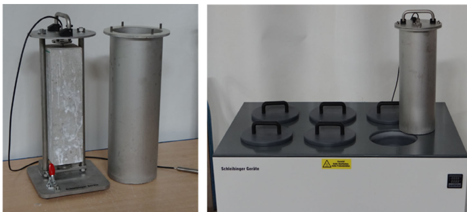
Figure 12. Specimen (75 mm × 75 mm × 280 mm) in a measurement frame and the container (left), and benchtop reactor for six specimen containers (right). Adapted with permission. [87] Copyright 2019, Ernst & Sohn.
