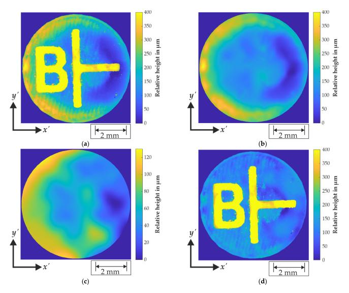
**Figure 5.** (a) Part surface extracted by thresholding algorithm. (b) Reconstructed part surface after removal of registration landmarks. (c) Reconstructed surface from lowest pores in the transition zone (between sections 5 and 6) at an approximately average specimen height of 10.7 mm. (d) Part surface after application of deformation adjustment function extracted by thresholding algorithm.
