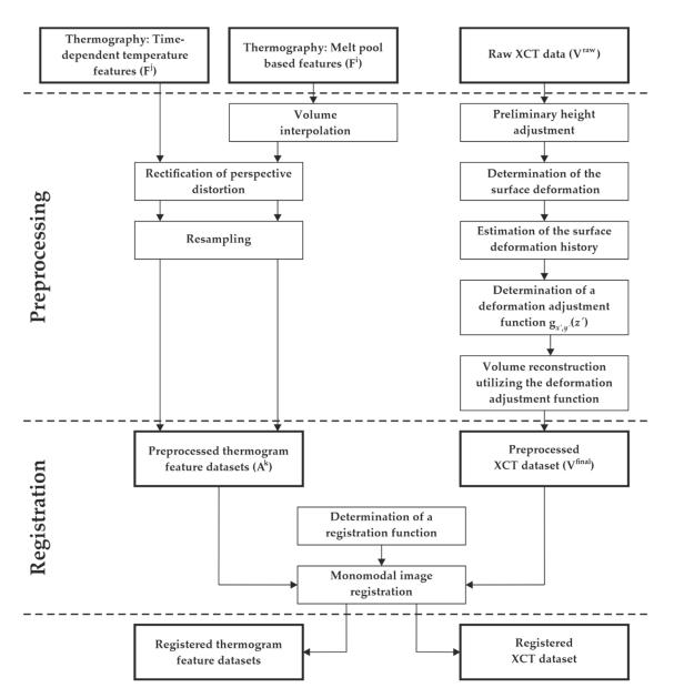
**Figure 2.** Schematic overview the processing steps for the registration of thermographic and XCT datasets. The dashed lines indicate which steps correspond to the data preprocessing and which correspond to the registration. Datasets are indicated by bold frames.
