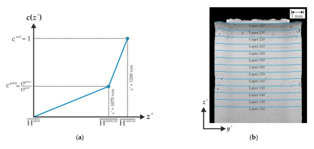
**Figure 6.** (a) Qualitative illustration of the linear sectional fit for the determination of the compression factor c. (b) Cross-sectional slice of the XCT data at a depth of 3.5 mm. The height deviations corresponding to the manufacturing layers calculated from  $g_{x',y'}(z')$  are depicted as blue lines.
