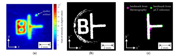
**Figure 8.** (a) Sum of temperature image from the raw 4D thermogram dataset. (b) x'-y' slice of  $V^{\text{bin}}$  at a height of z' = 1205 vox. (c) Extracted and processed cross labels from (**a**,**b**) after the spatial registration was performed. Shown here is a monomodal translation registration with a quality of 0.958 calculated by the MATLAB Registration Estimator Toolbox. White areas correspond to overlapping area, while pink and green correspond to deviating areas.
