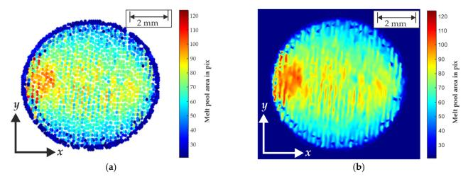
**Figure 3.** Preprocessing of thermogram feature data (here: melt pool blob size) of layer 59. (a) Incremental data points of melt pool blob size containing image distortion. (b) Rectified and resampled thermogram with an adjusted scale of  $10 \,\mu$ m/pix.
