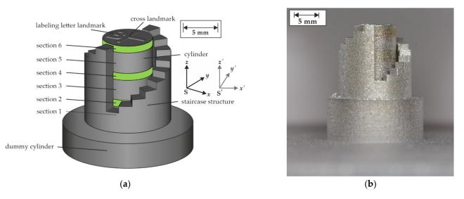
Figure 1. (a) Specimen design including staircase structure, top surface cross landmark, labeling letter landmark, dummy cylinder, and the introduced coordinate systems S and S'. The green areas mark sections that were manufactured using increased VED. In this view, section 1 is hidden behind the staircase which is indicated by the dashed line. (b) Manufactured specimen on dummy cylinder. Adapted from Ref. [28].
