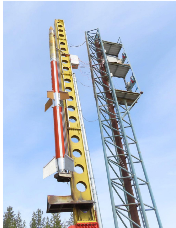
Fig. 11. MAPHEUS-11 vehicle during test countdown. Two-stage solid propellant engine (orange), and several experiment units (golden) stacked on top. The vehicle has a total length of approximately 12 m and carries 300 kg of scientific payload to an apogee of 250 km, allowing over 6 min of microgravity.
