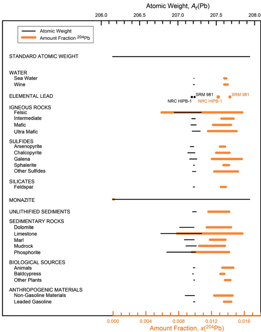
Fig. 6: Variation in atomic weight (black lines) of lead, A_r(\text{Pb}) , with amount fraction (orange lines) of ^{204}\text{Pb} , x(^{204}\text{Pb}) , of selected lead-bearing materials. Because lead has four isotopes whose variations are not mass-dependent, the changes in the A_r(\text{Pb}) and x(^{204}\text{Pb}) values are not superimposed. Each horizontal line spans the minimum and maximum values observed for the corresponding class of materials (data from [16]).
