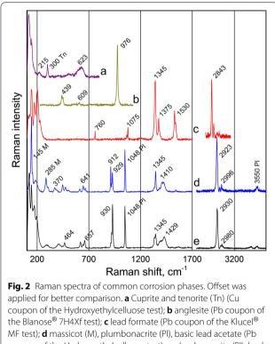
coupon of the Hydroxyethylcelluose test); **e** plumbonacrite (PI), lead acetate trihydrate (Pb coupon of the Hydroxyethylcelluose test)
