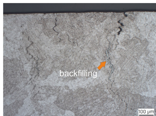
Figure 12. Solidification cracks and indicated backfilling in the cross-sections of the CrMn alloy (etchant LB I + 2% Nital) E = 14 \text{ kJ cm}^{-1} , v_s = 1.8 \text{ mm s}^{-1} .
