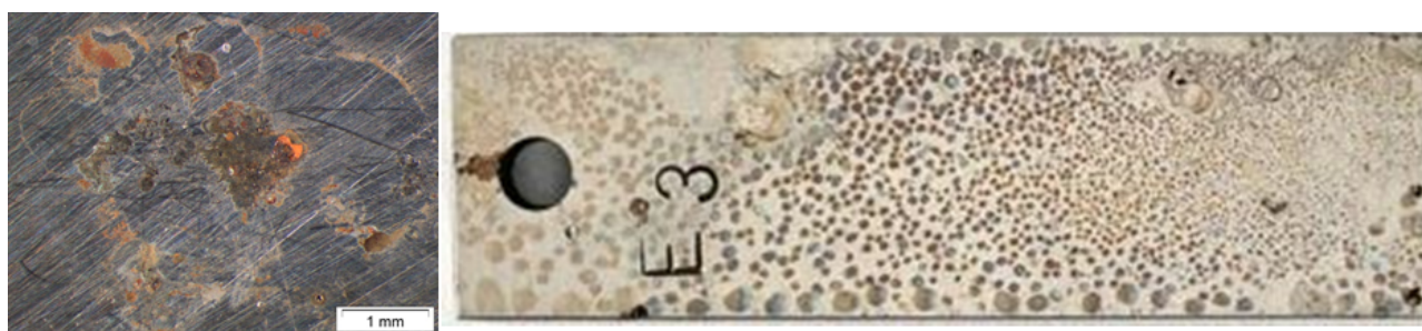
Figure 1. Left: SEM micrographs (8000 h at 60 °C/100 bar exposed to water-saturated supercritical CO 2 ) of the corrosion layer formed on X5CrNiCuNb16-4 with ellipsoidal peculiarity on hardened and tempered at 670 °C. Reprinted with permission from [16]. 2021 MDPI, A. Pfennig.
