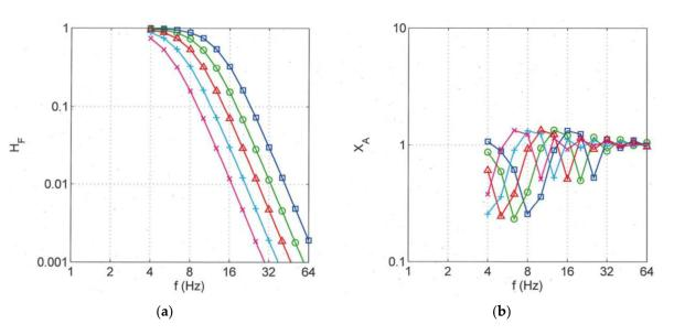
**Figure 3.** Spectra for the calculation of a standard ballast track with varying track support stiffness, (a) filter function of the track force, (b) axle-sequence spectrum of two axles of a bogie, train speed  $\times$  63, + 80,  $\Delta$  100,  $\bigcirc$  125, and  $\Box$  160 km/h.
