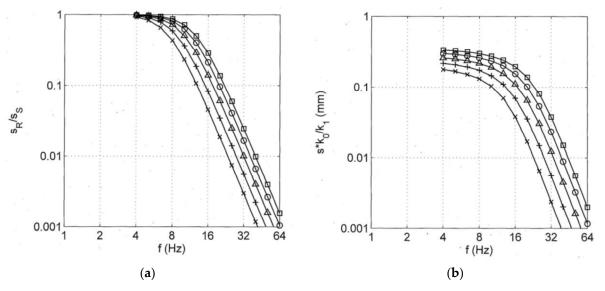
**Figure 5.** Transfer functions for the track filtering (**a**) of geometric track bed errors, and (**b**) of a stiffness variation, ballast tracks with different under-sleeper pads with stiffness of  $k_P = \times 10, + 20, \Delta 40, \bigcirc 80$ , and  $\Box 160 \ 10^6 \ N/m$ .
