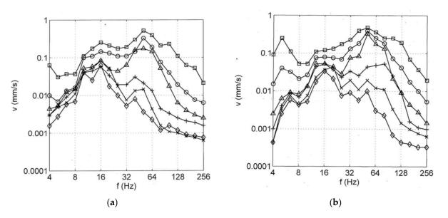
**Figure 1.** Train induced ground vibration, (**a**) at site N, (**b**) at site H, at distances  $x = \Box 3, \odot 5, \Delta 10, + 20, \times 30, \text{ and } \Diamond 50 \text{ m } [20].$
