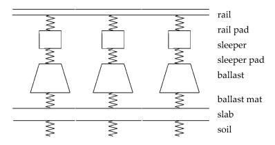
**Figure 2.** Track model consisting of rail, rail pad, sleeper, sleeper pad, ballast, ballast mat, ballast plate and continuous soil.
