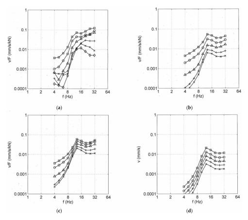
**Figure 9.** Transfer functions for the soil at site W, distances  $x = \Box 3$ ,  $\bigcirc 5$ ,  $\Delta 10$ , + 20,  $\times 30$  m, (a) measured from hammer impact, (b) calculated for a point load, (c) calculated for a standard train load; (d) response to constant train loads between 0.15 and 1 kN per one-third octave band representing train speeds of  $v_T = \Box 160$ ,  $\bigcirc 125$ ,  $\Delta 100$ , + 80, and  $\times 63$  km/h.
