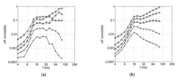
**Figure A1.** Transfer function of a soil with  $v_{S1} = 125$  m/s,  $v_{S2} = 350$  m/s, h = 4 m, D = 2.5% at distances  $x = \Box 4$ ,  $\bigcirc 8$ ,  $\Delta 16$ , + 32,  $\times 64$  m, (**a**) exact, (**b**) approximated solution.
