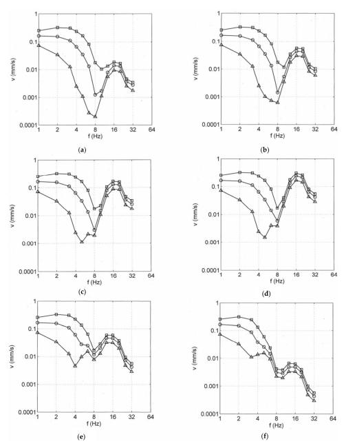
**Figure 7.** Train passage with  $v_T = 160$  km/h over an irregular track and a soil with  $v_S = 200$  m/s, irregularity  $q = (\mathbf{a}) 3\%$ , (**b**) 10%, (**c**) 30%, (**d**–**f**) 50%, track stiffness (**a**–**d**) *EI* ballast track, (**e**) 10 *EI*, (**f**) 100 *EI* slab track, one-third of the octave band spectrum at distances  $x = \Box 3$ ,  $\bigcirc 5$ ,  $\Delta 10$  m.
