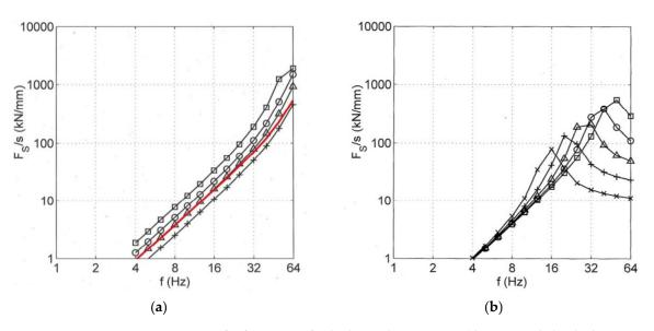
**Figure 4.** Transfer functions of vehicle–track interaction (dynamic axle loads due to irregularities) (a) for different wheelset masses  $m_W = +1000$ ,  $\Delta 1500$ ,  $\bigcirc 2000$ , and  $\Box 3000$  kg, — 1500 kg with  $H_T(f) = 1$ , and (b) for different under-sleeper pads with stiffness of  $k_P = \times 10$ , + 20,  $\Delta 40$ ,  $\bigcirc 80$ , and  $\Box 160 \times 10^6$  N/m.
