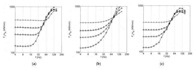
**Figure A2.** Dynamic stiffness of standard ballast track on soils with  $v_S = \Box 100$ ,  $\bigcirc 150$ ,  $\triangle 200$ , + 300 m/s, (**a**) wavenumber domain method with continuous soil, (**b**) with approximated Winkler soil, (**c**) boundary-element/finite-element method.
