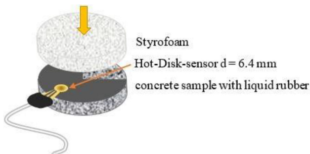
Fig. 4 Setup of the TSP method with the Hot-Disk sensor in one-sided configuration
