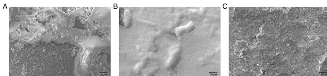
Figure 9. SEM images of binary and ternary zinc coatings after 21 days of artificial aging, top view. A) ZnFe/ZnFeMo coating without post-treatment. B) ZnFe/ZnFeMo coating + passivation. C) ZnNi coating without post-treatment.
