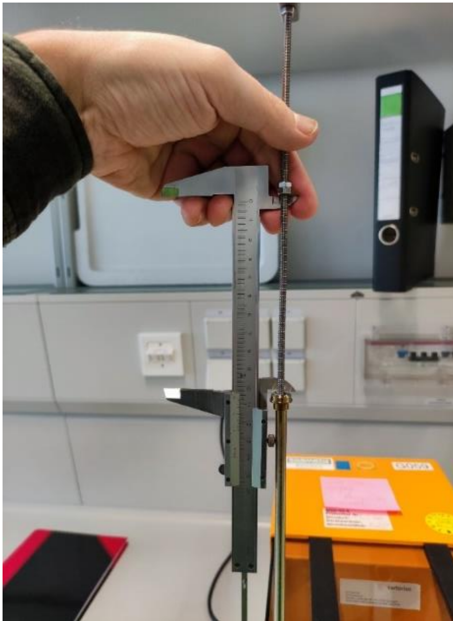
Figure S17. Measurement of the sample's volume into the HPVA analysis cell.
