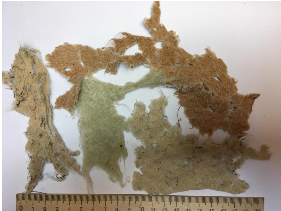
Figure 1.2. Fragments of nonwoven geotextile (PP, PET). All pieces are not fresh; they were a long time in natural conditions.
