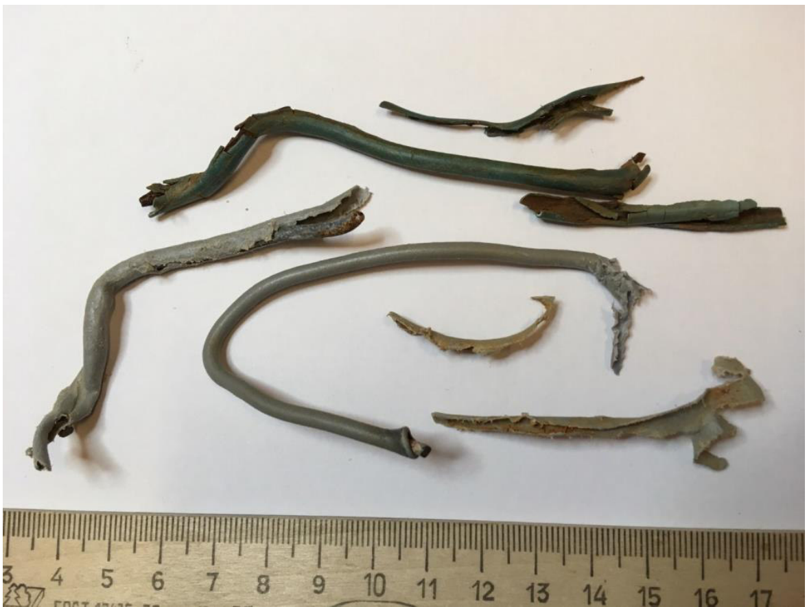
Figure 1.9. Usually, only fragments of plastic coating for gabion wire are present on the beach, but sometimes the pieces contain the wire (two pieces in the figure).
