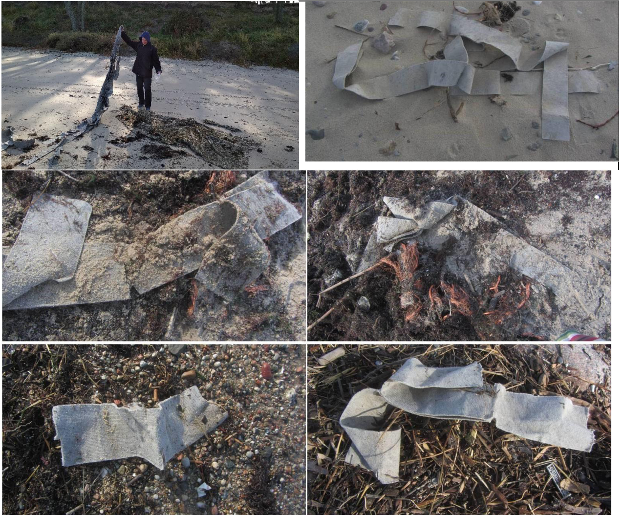
Figure 1.16. Examples of the geocell fragments on the beaches of the Kaliningrad Oblast, Russia.
