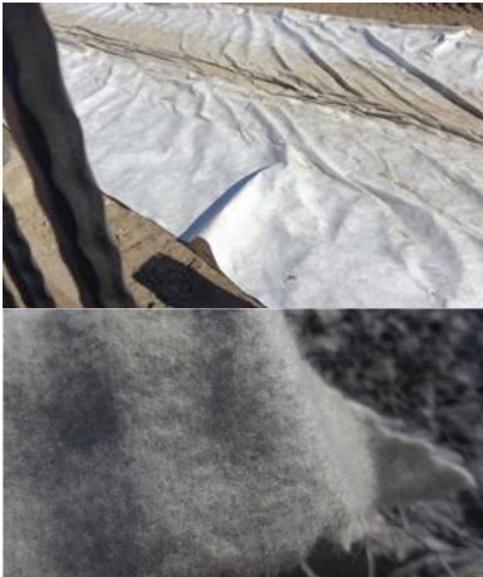
Figure 1.1. Nonwoven geotextile (PP, PET) is used in coastal protection constructions.
