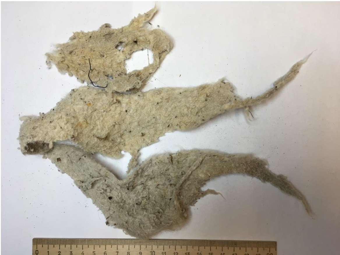
Figure 1.6. The Fragment of white nonwoven geotextile (PP, PET) ). Pieces are not fresh; they were a long time in natural conditions.
