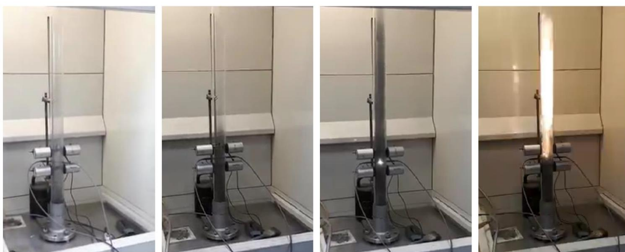
Fig. 4. Experimental observation of the flame propagation of an aluminium sample
