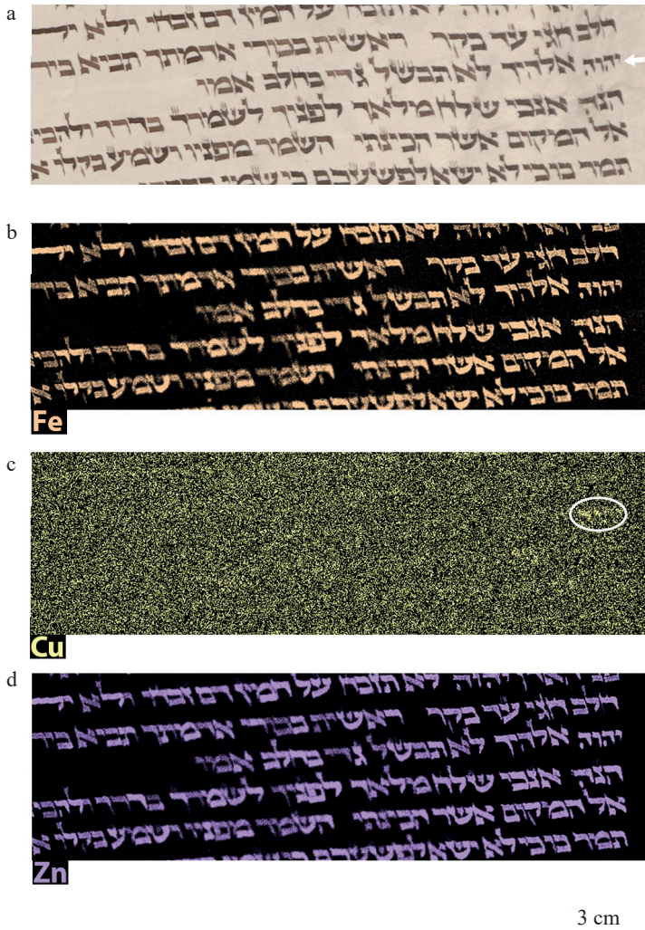
Fig. 6. Portion of sheet 19 column 1 Exodus 23,19-20; (a) image of the scanned area; (b) map of iron (Fe); (c) map of copper (Cu), with God's name is marked with a white ellipse and with an arrow in the photograph; (d) map of zinc (Zn).
