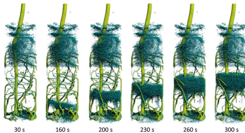
Figure 3. Visualization of the water uptake by the root system of a lupine by dynamic neutron tomography after the injection of 4 mL deuterated water ( D_2O ) through the bottom. The time series ( 30\text{ s} \leq t \leq 300\text{ s} ) shows the ascending front of water ( H_2O ) moving upwards as it is being displaced by the injected deuterated water. The repetition time for the tomograms is just 10 s [48]. Copyright: Christian Tötze (University of Potsdam, Germany), published in [48]. The image is included in the article's Creative Commons license: http://creativecommons.org/licenses/by/4.0/ .
