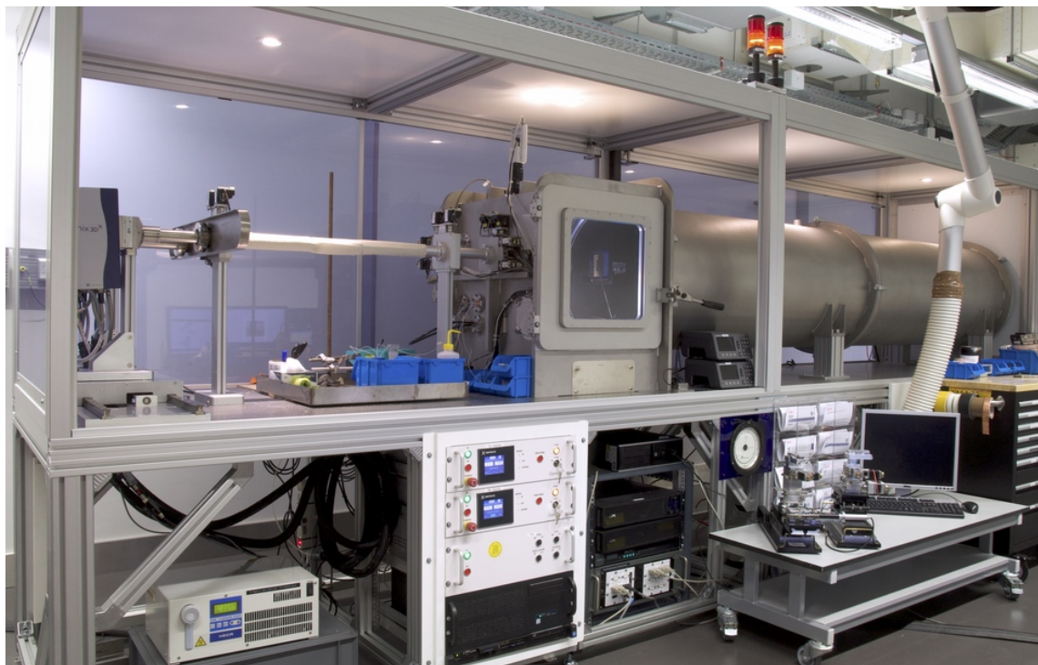
Figure 1. The MOUSE instrument in its current form, with outer dimensions of 5 \times 1.5 \times 2 m (Length \times Width \times Height).
