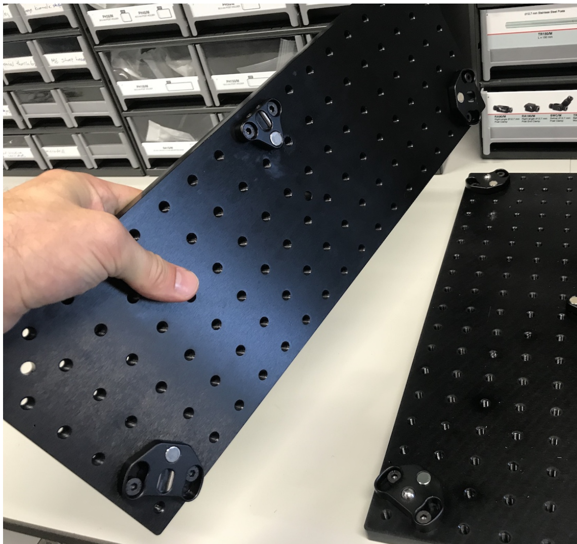
Figure 9. The standard, “M-sized” M-sized”, MOUSE sample environment mounting plate with three kinematic feet attached.
