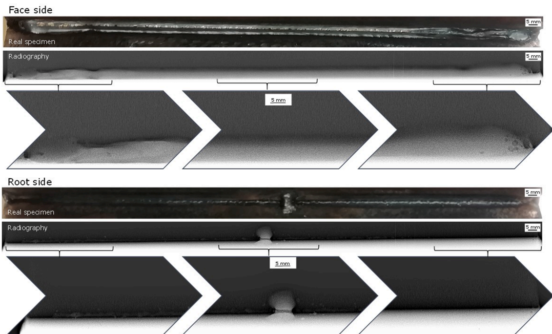
Fig. 16. X-Ray test at face side and root side in welded T-joint specimen of Test 10.
