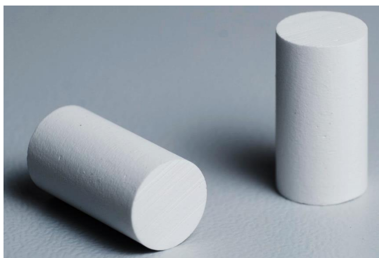
Figure 2. Close-up of the raw cylinder based on the partially sintered borosilicate glass VitraPOR 5, diameter 8 mm, length 15 mm, volume 0.75 mL.
