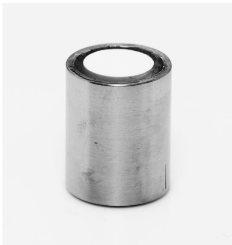
Figure 3. Raw cylinder, glued into a titanium tube, outer diameter 12 mm, inner diameter 10 mm (details see Supplementary Materials).
