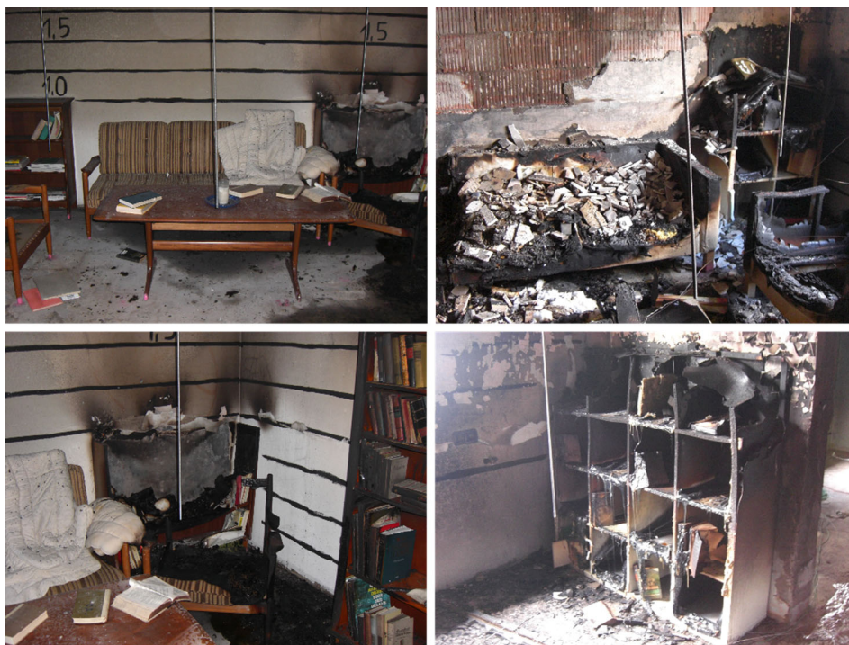
FIGURE 12 Living room with older furniture (left), with modern furniture (right) after the fire tests [Colour figure can be viewed at wileyonlinelibrary.com ]
