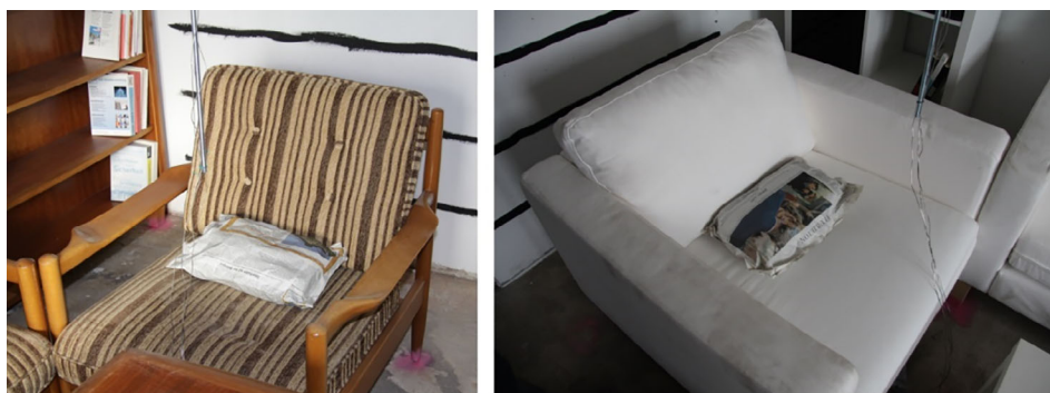
FIGURE 5 First burning item: upholstered chair with paper cushion, left hand side: older chair, right hand side: modern chair [Colour figure can be viewed at wileyonlinelibrary.com ]
