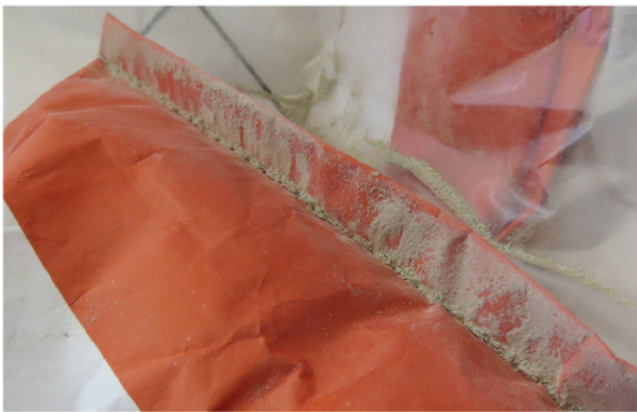
FIGURE 9 Release of a UN No. 3077 substance—leaking stitched closure of a 5M2 bag (Police North Rhine-Westphalia Münster)
