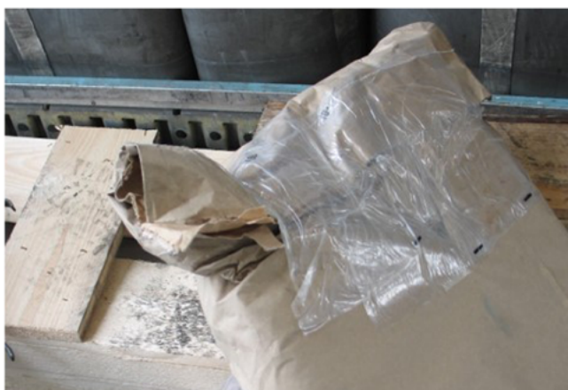
FIGURE 14 Release from the closure of a paper bag that is only provisionally sealed with adhesive tape (Police North Rhine-Westphalia Münster)
