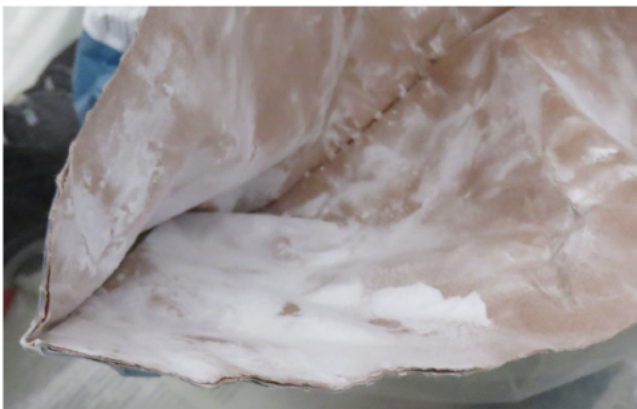
FIGURE 10 Release of a UN No. 3077 substance—leaking stitched closure of a 5M2 bag (Police North Rhine-Westphalia Münster)
