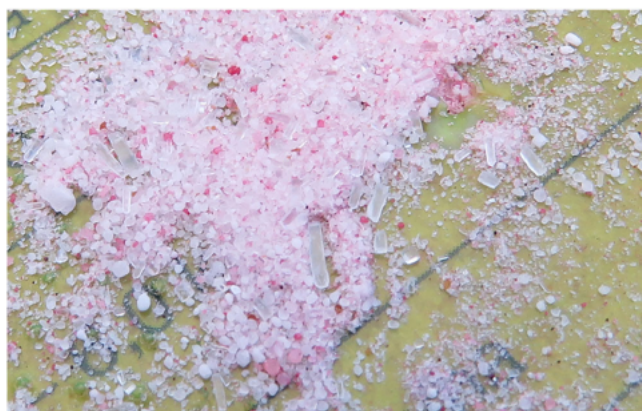
FIGURE 1 Release of a UN No. 1486 substance from the micro-perforations of a 5H4 bag (Police North Rhine-Westphalia Münster)
