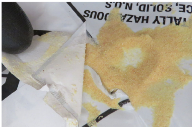
FIGURE 13 Release of a UN No. 3077 substance—provisionary closed damaged area (adhesive tape) in a 5H4 bag (Police North Rhine-Westphalia Münster)
