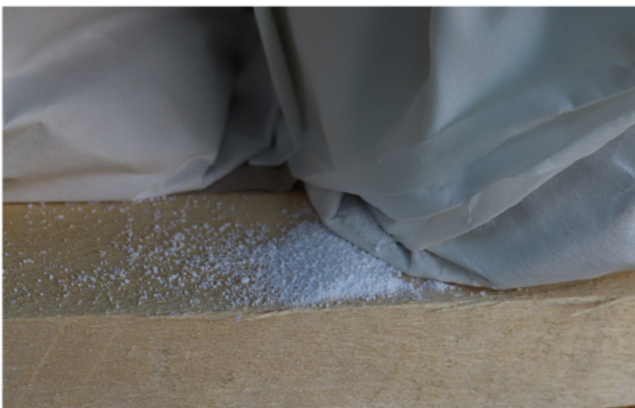
FIGURE 4 Release of a UN No. 3261 substance—leaking pasted join of a 5M2 bag (Police North Rhine-Westphalia Münster)
