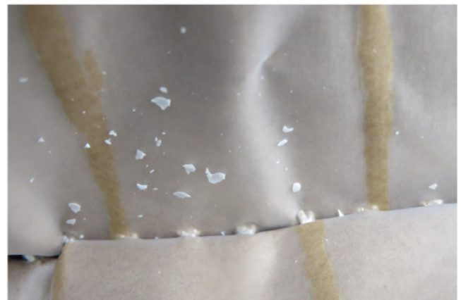
FIGURE 7 Release of a UN No. 3077 substance—leaking stitched closure of a 5M2 bag (Police North Rhine-Westphalia Münster)
