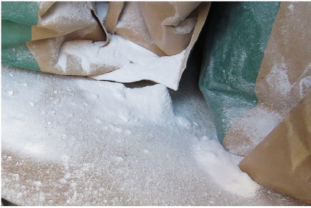
FIGURE 3 Release of a UN No. 3077 substance—leaking internal sleeve valve of a 5M2 bag (Police North Rhine-Westphalia Münster)
