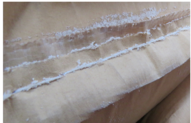
FIGURE 12 Release of a UN No. 3077 substance—leaking stitched join of a 5M2 bag (Police North Rhine-Westphalia Münster)
