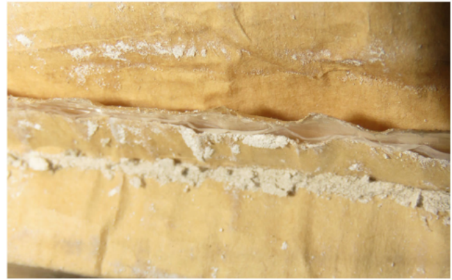
FIGURE 11 Release of a UN No. 3077 substance—leaking stitched join of a 5M2 bag (Police North Rhine-Westphalia Münster)
