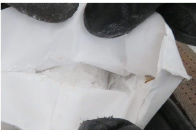
FIGURE 5 Release of a UN No. 3077 substance—leaking pasted closure of a 5M2 bag (Police North Rhine-Westphalia Münster)
