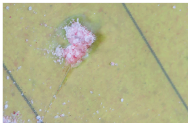
FIGURE 2 Release of a UN No. 1486 substance from the micro-perforations of a 5H4 bag (detail) (Police North Rhine-Westphalia Münster)
