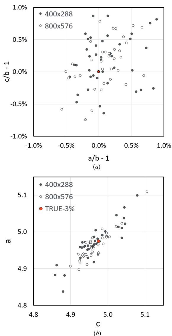
Figure 7 Analysis of 41 patterns of rhombohedral corundum ( \text{Al}_2\text{O}_3 ) collected with a resolution of 400 \times 288 pixels and 34 patterns of 800 \times 576 pixels. (a) Displays the deviation of a/b and c/b from 1, whereas (b) presents the absolute lattice parameters derived for a and c ( b as well as \alpha , \beta and \gamma are not shown). The red dot shown in (b) and labelled TRUE-3% marks a 3% shorter basis vector length than that typical for corundum ( a = 5.1288 \text{ \AA} ).
