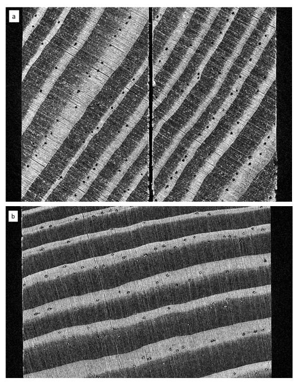
Fig.2.16 X-ray micro-CT images of the transverse section of Scots pine wood (20 mm x 15 mm) treated with NMF (a) before leaching (b) after leaching.
