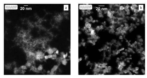
Fig.2.4 High-angle annular dark field-STEM image of MgF<sub>2</sub> and CaF<sub>2</sub> nanoparticles from (a) one-step sol in ethylene glycol as solvent (b) combined from two sols, one in ethylene glycol and the other in lactic acid.
