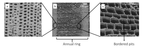
Fig. 1.6 Cross-cut section of Scots pine in back-scattered electron image showing tracheids (a) latewood tracheids (b) annual ring (c) earlywood tracheids with bordered pits. Image created by S. M. Usmani.
