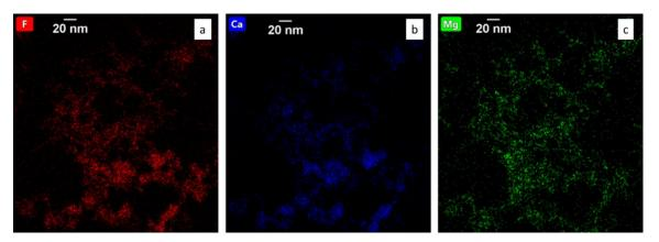
Fig.2.5 Elemental map of (a) Fluorine (b) Calcium (c) Magnesium in MgF<sub>2</sub> and CaF<sub>2</sub> nanoparticles synthesized together in one sol with ethylene glycol as solvent.
