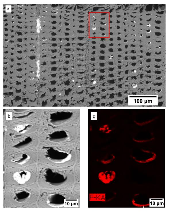
Fig.2.14 Transverse section of Scots pine wood treated with NMFs. BSE image showing aggregates of NMF in rays and latewood cell lumina (a) low and (b) high resolution. (c) EDX map of fluorine (red) in the latewood cell lumina.
