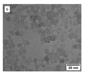
Fig. 2.3 HR-TEM image of MgF<sub>2</sub> and CaF<sub>2</sub> nanoparticles (a) synthesized together in one sol with ethylene glycol as solvent (b) combined from two sols, one in ethylene glycol and the other in lactic acid.
