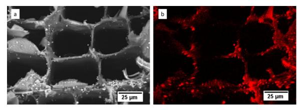
Fig.2.15 Transverse section of Scots pine wood treated with NMF. (a) BSE image showing aggregates of NMF scattered in earlywood cell lumina (b) EDX color map of fluorine (red) in earlywood cell lumina.
