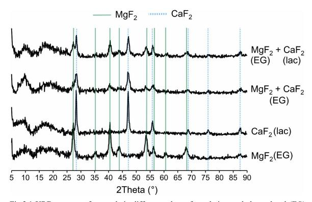
Fig.2.1 XRD patterns of xerogels in different solvent formulations, ethylene glycol (EG) and lactic acid (lac). The vertical lines are the reference peaks from MgF<sub>2</sub> (PDF 41-1443) and CaF<sub>2</sub> (PDF 35-0816). 109
