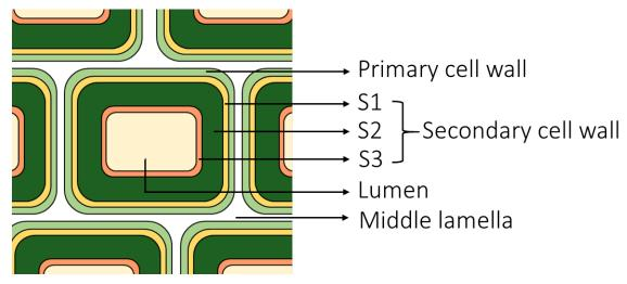
Fig.1.4 Schematic representation of wood cell wall components. Image created by S. M. Usmani.
