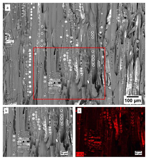
Fig.2.12 Radial longitudinal surface of Scots pine wood treated with NMF. BSE image showing bordered pits and ray tracheids (a) low and (b) high resolution. (c) EDX map of fluorine (red) in the ray tracheids and bordered pits.
