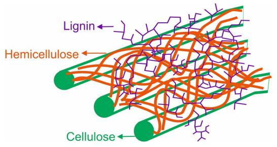
Fig.1.3 Schematic representation of the interaction of wood polymers in the secondary cell wall. Image created by S.M. Usmani.
