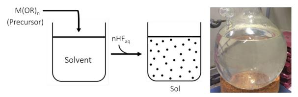
Fig.1.11 Schematic of fluorolytic sol-gel synthesis and an example of a clear CaF<sub>2</sub> sol (right), where M(OR) = metal alkoxide and n = metal valence. Image created by S. M Usmani.
