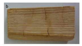
Fig.1.8 Wood specimens damaged by (a) *C. puteana* and (b) *R. placenta*. Image taken by S. M. Usmani.
