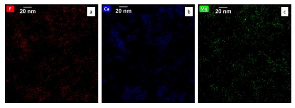
Fig.2.6 Elemental map of (a) Fluorine (b) Calcium (c) Magnesium in MgF<sub>2</sub> and CaF<sub>2</sub> nanoparticles combined from separately synthesized sols of MgF<sub>2</sub> in ethylene glycol and CaF<sub>2</sub> in lactic acid.
