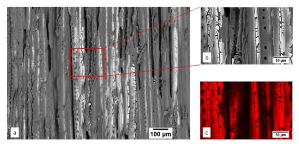
Fig.2.11 Tangential longitudinal surface of Scots pine wood treated with NMFs. BSE image showing bordered pits and longitudinal tracheids at (a) low and (b) high resolution. (c) EDX map of fluorine (red) in the longitudinal tracheids and bordered pits.
