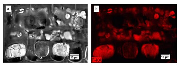
Fig.2.13 Ray tracheids of Scots pine wood treated with NMFs. (a) BSE image showing aggregates of NMF in ray tracheids (b) EDX map of fluorine (red) in the ray tracheids.
