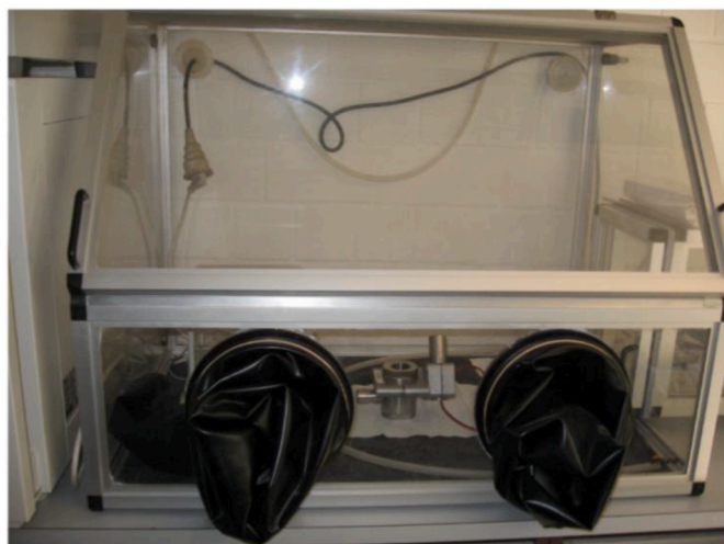
Fig. 2. N 2 -inertized glove box with test reactor.
