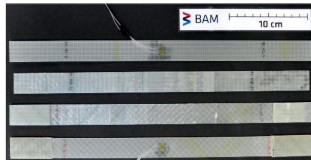
Figure 7. Exemplary specimens of all four types tested in this study, from top to bottom: control \pm 45^\circ , repaired \pm 45^\circ , repaired 0/90^\circ , and control 0/90^\circ .
