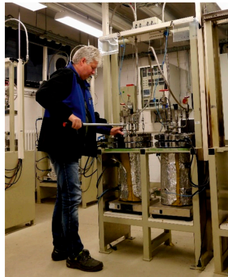
Figure 1. Schematic view of autoclave test equipment (left), closing the cover plate of the autoclaves (test rig with two autoclaves).
