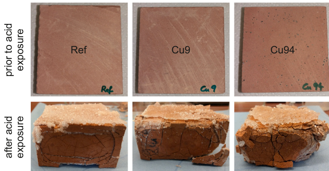
Fig. 2. Visual appearance of specimen before (top view) and after (side view) the exposure to H_2SO_4 .
