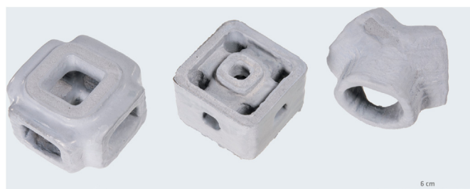
Fig. 1. Examples of manifolds produced from lithium aluminate/microsilica slurries with the LIS-process described by Hlaváček et al. [25].
