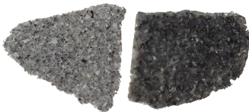
FIGURE 1 Thick section samples after alkali attack (KOH), without (left) and with (right) exposure to aluminium solution
