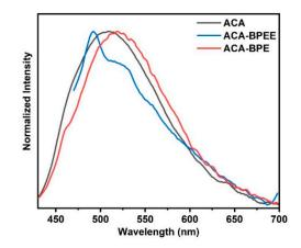
**Figure 5.** Solid-state photoluminescence spectra of ACA ( $\lambda_{ex} = 420 \text{ nm}$ ), ACA-BPEE ( $\lambda_{ex} = 450 \text{ nm}$ ), and ACA-BPE ( $\lambda_{ex} = 420 \text{ nm}$ ).
