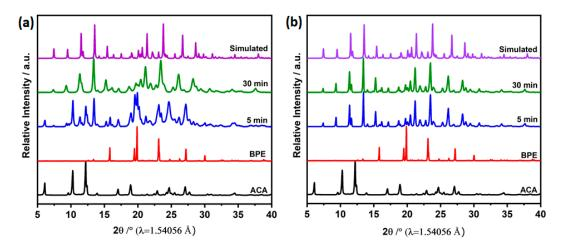
**Figure 3.** PXRD patterns of 9-anthracenecarboxylic acid (ACA), 1,2-bis(4-pyridyl)ethane (BPE), and the mechanochemically synthesized ACA-BPE cocrystal with respect to different time intervals with (**a**) neat grinding (NG) and (**b**) liquid-assisted grinding (LAG) with MeOH.
