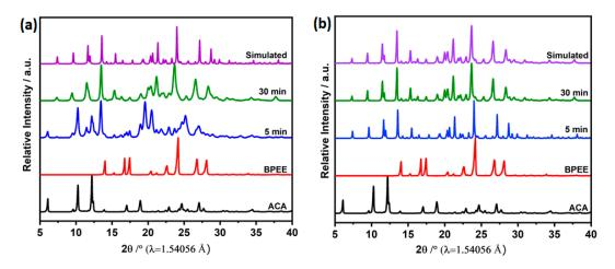
**Figure 2.** Powder X-ray diffreaction (PXRD) patterns of 9-anthracenecarboxylic acid (ACA), 1,2-bis(4-pyridyl)ethylene (BPEE), and the mechanochemically synthesized ACA-BPEE cocrystal with respect to the different time intervals with (**a**) neat grinding (NG) and (**b**) liquid-assisted grinding (LAG) with MeOH.
