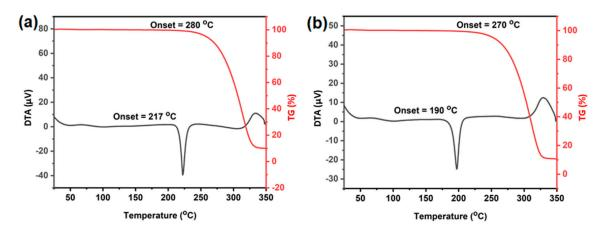
**Figure 4.** Differential thermal analysis-thermogravimetric (DTA-TG) measurements of (**a**) ACA–BPEE and (**b**) ACA–BPE, respectively. The DTA signals (black) of the cocrystal at the onset 217 °C (for ACA–BPEE) and 190 °C (for ACA–BPE) can be assigned to the melting of the cocrystals, and after that, the complete mass losses are observed in the TG analysis (red).
