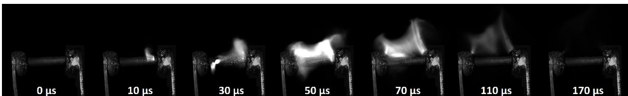
Fig. 11. Full ignition procedure of a surface-gap spark, burning duration of less than 0.17 ms
