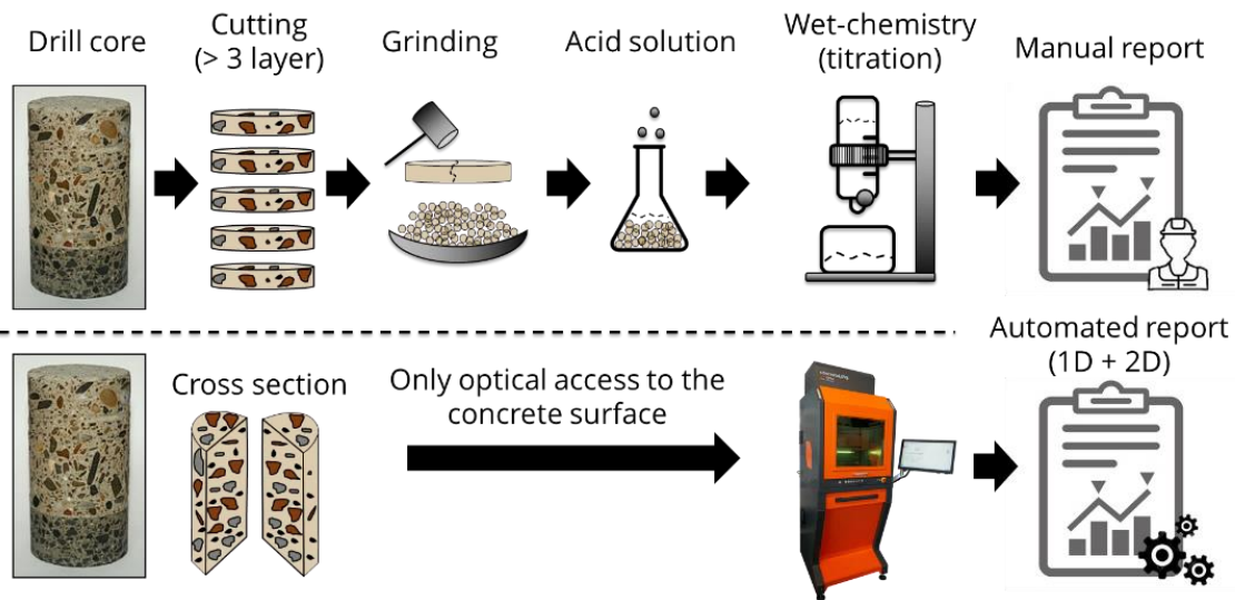
Figure 5. Sample preparation steps for the standard procedure compared to LIBS for concrete analysis.
