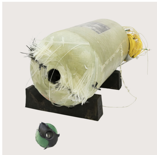
Fig. 6. Pressure vessel after burst. The tank failed in the dome with connection port, which was completely ejected from the pressure vessel body.
