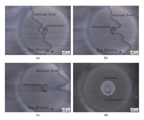
**Figure 11.** Temporal course of fluid flow around glass lens in tribocontact and building of meniscus. (a) Fluid front approaching the tribocontact; (b) fluid front passing by the tribocontact; (c) fluid filling the channels behind the tribocontact and (d) building meniscus started at the contact of the lens with the sample.
