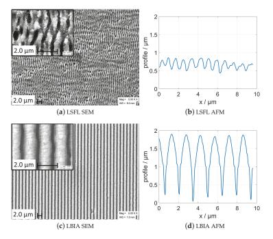
**Figure 2.** Laser-based surface modification using the LSFL and LBIA method. SEM image of LSFL (**a**) reveals a mostly vertical orientation of the structes and the corosponding AFM profile (**b**) shows the height profile. Structures fabricated by LBIA show a high homogeneity in the SEM image (**c**) and the AFM profile (**d**).
