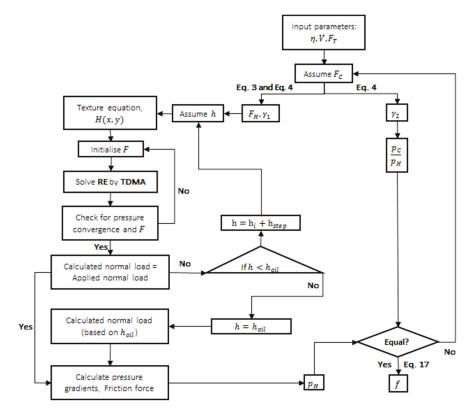
Figure A1. Flowchart of mixed lubrication under starved lubrication condition.
