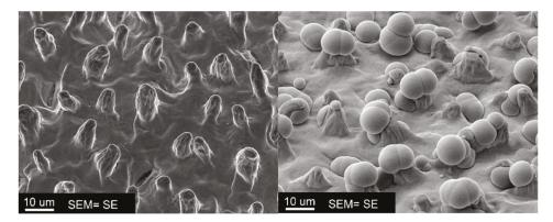
Figure 4. Multi-scale surface textures on nickel created by replicating the natural surface of the lotus leaf and a subsequent electrodeposition step. Adapted from [46].
