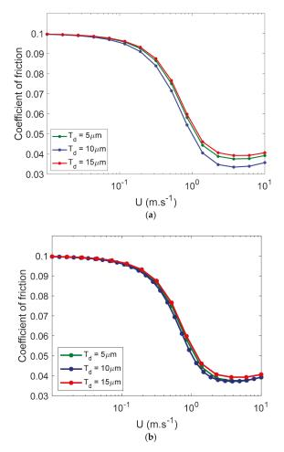
**Figure 11.** Stribeck curves as a function of texture depth for grooves when the lubrication is: (a) Non-starved, (b) starved, and  $h_{oil} = 10 \,\mu\text{m}$ .
