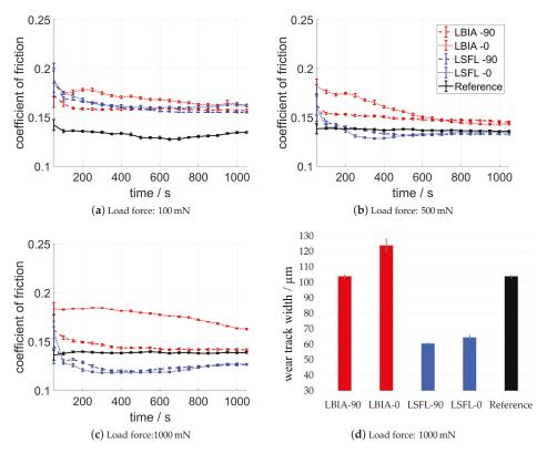
**Figure 7.** Tribological evaluation using tungsten carbide triboballs in a lubricated environment. Temporal evolution of the coefficient for a load force of 100 mN (a), 500 mN (b), and 1000 mN (c). Wear track width on the 100Cr6 substrate after after 1000 s test duration using a load force of 1000 mN and tungsten carbide triboballs (d).
