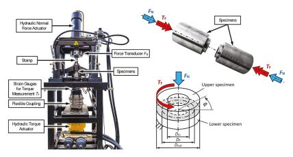
Figure 4. Test bench assembly and standard procedure developed at IKAT (Chemnitz University of Technology) to analyze the performance of frictional contacts [33,34].
