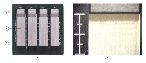
**Figure 7.** Experimental investigation of fluid transport in laser textured surfaces. (**a**) Specially designed sample with different regions. 1: Reservoir, 2: Laser surface textures, 3: mm-scale (500 µm per bar); (**b**) fluid front propagating in laser textures at a distance of 500 µm.
