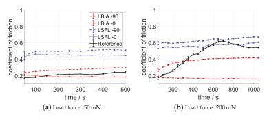
Figure 5. Temporal evolvement of the coefficient of friction using tungsten carbide triboball without lubrication for a load force of 50 mN (a) and 200 mN (b).
