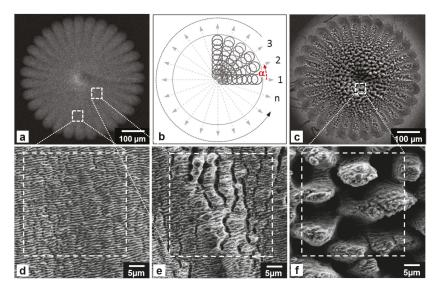
**Figure 6.** SEM micrographs showing ripple (**a**) and cone-like protrusion (CLP) (**c**) surface textures produced on stainless steel; the direct-write scanning procedure for the radial matrices as used for tightly mapping a variable set of pulse overlaps (**b**); magnified view on low spatial frequency LIPSS (LSFL) (**d**), micro grooves and spikes (**e**) as well as CLPs (**f**) originating at low and high peak fluence pulses of 0.7 J/cm<sup>2</sup> and 3.7 J/cm<sup>2</sup>.
