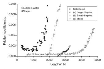
**Figure 5.** Coefficient of kinetic friction (COF) versus load curves in order to determine the critical load for an untextured reference as well as single-scale (large and small dimples) and multi-scale surface textures (mixed). Adapted from [91].
