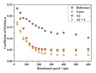
**Figure 7.** COF versus rotational speed for an unpolished reference, a purely laser-textured sample (laser), a solely micro-coined sample (A2) and the respective multi-scale samples combining direct laser interference patterning (DLIP) and micro-coining. Adapted from [72].
