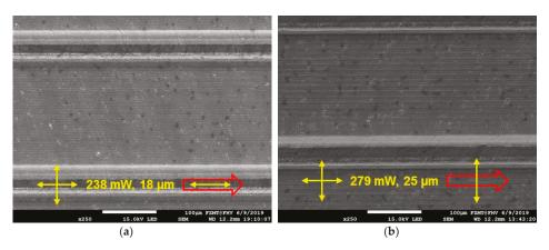
**Figure 5.** Surface quality after laser ablation: (**a**) reduced laser power and polarization of final scan cycle parallel to scan direction; (**b**) increased laser power and number of scans, but polarization of the last scan cycle perpendicular to the scan direction.
