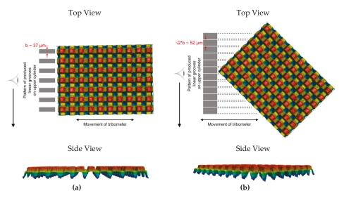
**Figure 15.** Explanation of (**a**) presence of visible linear grooves (width of grooves = sides of plateaus ~37  $\mu$ m) on cylinders for the 3D-texture with an angle of 90° to the direction of motion and (**b**) near absence of visible linear grooves (width of grooves = diagonals of plateaus = ~52  $\mu$ m) on cylinders for the 3D-texture with an angle of 45° to the direction of motion.
