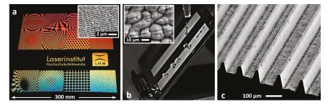
**Figure 2.** Laser made microscopic surface textures for mimicking natural functionalities on stainless steel: (a) rippled surface texture for optical effects; (b) multi-scale features imitating the hydrophobic and self-cleaning behavior of the lotus leaf and (c) riblets for skin friction drag reduction in turbulent flows inspired by shark's skin micro structure.
