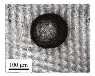
**Figure 3.** Multi-scale surface textures created by a combination of micro-coining and direct laser interference patterning. The bigger micro-coined textures have a diameter of 180  $\mu$ m and a depth of 43  $\mu$ m, whereas the cross-like laser pattern has a width of 6  $\mu$ m and a depth of 0.6  $\mu$ m. Adapted from [70].
