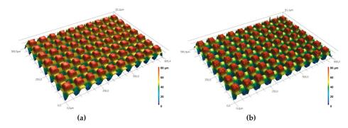
Figure 10. Typical topographies of two selected 3D surface microtextures produced on disc specimens: (a) first sample; (b) second sample.
