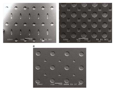
**Figure 2.** Multi-scale surface textures created by laser surface texturing using a pulsed Q-switched Nd:YAG laser with a power of 24 W and a pulse duration of 200 ns. The smaller textures (squares, triangles) have a side length of 250  $\mu$ m while the bigger circles have a diameter of 500  $\mu$ m. Adapted from [66].
