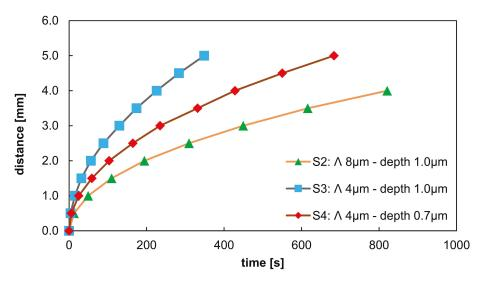
**Figure 8.** Quantitative results of flow behavior in different Direct Laser Interference Patterning (DLIP) textures (S2–S4). The sample introduced in Figure 7 was used to measure the distance of the fluid column in different channel-like textures as a function of time. The curves show Washburn-like behavior with the fastest transport in channels with smaller period and higher depth.
