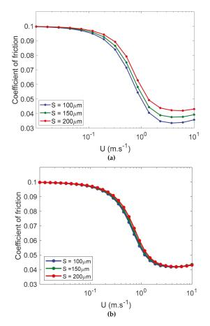
**Figure 13.** Stribeck curves as a function of cavity size (*S*) for grooves when the lubrication is: (a) Non-starved, (b) starved, and  $h_{oil} = 10 \ \mu\text{m}$ .
