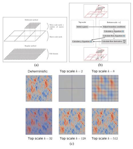
**Figure 18.** Overview of the multi-scale finite element method proposed by [233] to simulate hydrodynamic lubrication of large rough contact surfaces, which can be extended to deal with multi-scale textures. (a) Multi-scale mesh. (b) Multi-scale solution procedure. (c) Comparison between full deterministic and top-scale pressure distribution with different values.
