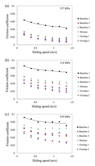
**Figure 6.** COF versus sliding speed for different reference cases (polished and single-scale textures) and different designs for multi-scale surface textures (mixture and overlapping textures) depending on the acting contact pressure (**a**) 157 MPa, (**b**) 314 MPa and (**c**) 470 MPa. The black baseline represents the polished reference surface, whereas baseline 2 and 3 stand for the single-scale surface textures. Adapted from [55].
