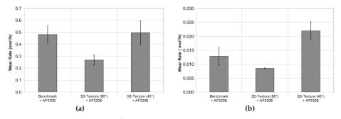
Figure 16. Average wear rate  $(mm^3/h)$  calculated from laser microscopy measurements after long-term tribological tests (2 h) of: (a) discs and (b) cylinders.
