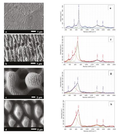
**Figure 8.** Raman analysis carried out on untreated stainless steel surface for reference purposes (**a**) as well as laser made ripple (**b**) and CLP (**c**,**d**) surface textures. The corresponding Raman signals detected following 473 nm laser excitation are presented on the right side of the figure (**e**–**h**).
