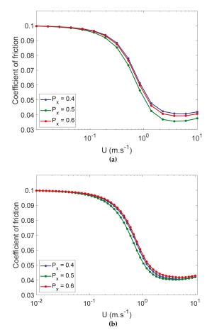
**Figure 16.** Stribeck curves as a function of texture pitch for chevrons when the lubrication is: (a) Non-starved, (b) starved, and  $h_{oil} = 10 \,\mu\text{m}$ .
