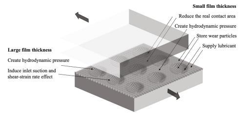
**Figure 19.** Schematic illustration of the possible mechanisms responsible for improved tribological performance of multi-scale surface textures. In this example, larger dimples with superimposed smaller cross-like textures are shown.
