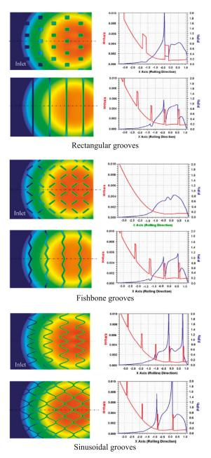
**Figure 13.** Deterministic simulations obtained with the fully coupled mixed-TEHL model proposed by Hu and Zhu. Sample cases with textured surfaces: rectangular (left), fishbone (middle) and sinusoidal (right) grooves with corresponding film thickness countors, centerline pressures, and normalized film thicknesses. Adapted from [118].
