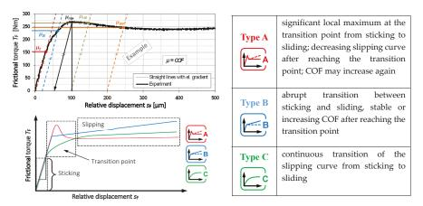
**Figure 5.** Exemplary illustration of the evaluation methods applied to determine the static COF. In the example (top, left), the stiffness lines are indicated by dashed lines to determine the respective COF's  $\mu_2$ ,  $\mu_{20}$  etc. Three types of friction can be distinguished depending on the torque progression curve schematically shown bottom, left. A detailed description of the different friction types is provided in the table on the right.
