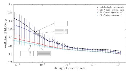
**Figure 9.** Experimental results from tribological evaluation of selectively structured samples. The Stribeck curves of three different samples with the same laser texture S1 ( $\lambda = 8 \mu m$ , depth = 1.5  $\mu m$ ) but with differently structured regions ("fully textured", "triboregion blank" or "triboregion only") are compared to the Stribeck curve of a polished reference sample.
