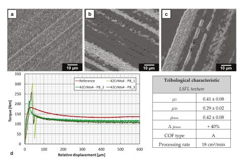
**Figure 10.** SEM micrographs showing the LSFL ripple texture (**a**) before and (**b**) after friction testing and (**c**) the rippled counter body surface after the friction test; the recorded slipping curves (**d**) and a summary of the tribological characteristic of LSFLs (table bottom, right) are presented.
