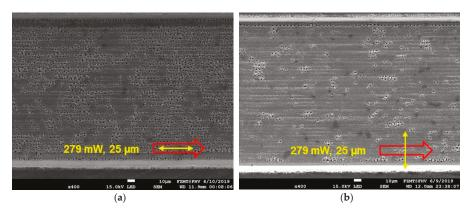
Figure 6. Surface quality after laser ablation without any polarization flipping: (a) polarization permanently parallel to scan direction; (b) polarization permanently perpendicular to scan direction.
