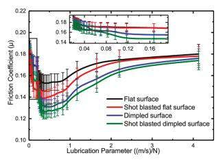
Figure 9. COF versus lubrication parameter for a flat surface, a shot-blasted sample, a dimpled sample, and a shot-blasted dimpled (i.e., multi-scale) surface. Adapted from [47].
