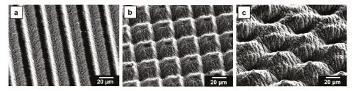
Figure 11. Deterministic surface textures made by ultrashort pulse laser processing under varied laser beam scanning procedures: (a) line pattern, (b) cross pattern and (c) alternating line and crosswise scanned laser beam.
