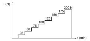
Figure 8. Schematic representation of the load-varying tribological tests used for the determination of the dynamic friction coefficients.
