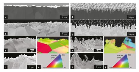
**Figure 7.** SEM micrographs recorded with the SE (**a**,**f**) and BSE detector (**b**,**g**); detailed micrographs (**c**,**d**,**h**,**i**) and electron back scatter diffraction (EBSD) mappings (**e**,**j**) to illustrate the depth of the laser affected zone.
