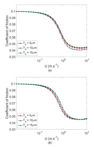
**Figure 12.** Stribeck curves as a function of texture depth for chevrons when the lubrication is: (a) Non-starved, (b) starved, and  $h_{oil} = 10 \,\mu\text{m}$ .
