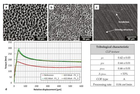
**Figure 9.** SEM micrographs showing the CLP texture (**a**) before and (**b**) after friction testing and (**c**) the fine grinded counter body surface after the friction test; the recorded slipping curves (**d**) and a summary of the tribological characteristic of CLPs (table bottom, right) are presented.
