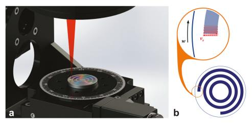
**Figure 1.** (a) Schematic of the laser treatment as a laser beam is scanned over a sample. (b) Details of laser patterning strategy: the laser beam is moving forth and back, while the sample is rotating by angular stage.
