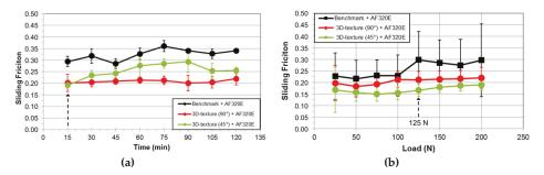
**Figure 13.** Average coefficients of friction measured: (a) during wear resistance tests (long-term tribological tests: 125 N, 2 h) and (b) during load-varying tests (short-term tribological tests: 25–200 N, 5 min. per load level) (Figure 13 = partial combination of Figure 12a,c).
