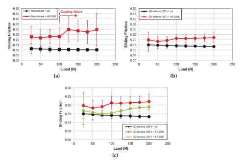
**Figure 12.** Sliding coefficients of friction as a function of applied load: (**a**) benchmark with oil or antifriction coating AF320E, (**b**) 3D microtexture (90°) with oil or antifriction coating AF320E, and (**c**) comparison of all 3D microtexture results (note: different scales for y-axis).
