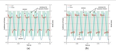
**Figure 9.** Example of raw signals obtained using FSA (high frequency signal acquisition) used for the calculation of both static and dynamic coefficients of friction (example shown: (a) benchmark (untextured samples) with oil at  $F_N$  = 175 N and (b) 3D microtexturing with oil at  $F_N$  = 175 N).
