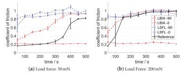
**Figure 3.** Temporal evolvement of the coefficient of friction using 100Cr6 triboball without lubrication for a load force of 50 mN (**a**) and 200 mN (**b**).
