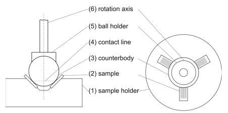
**Figure 2.** Experimental setup for tribological evaluation. A side view on the left-hand side and a top view on the right-hand side shows the important components of the setup and the contact line (**4**) on the rotating ball (**3**).
