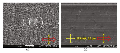
**Figure 7.** Micrographs: (a) LIPSS intersections perpendicular to their orientation where small pinhole formation starts; (b) same laser procedure as in Figure 5b but with enlarged scale (polarization of the last scan cycle was perpendicular to the scan direction).
