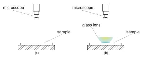
**Figure 1.** Experimental setup for fluid transport evaluation. In (**a**) the setup for the fluid transport evaluation inside the laser textures is shown. The fluid propagation in the channel-like textures is observed via a microscope from the top. In (**b**) the setup for the lens experiments is illustrated. The transparent glass lens is a substitute for the tribological counterpart and allows fluid flow analysis at the transition region between channels and tribocontact.
