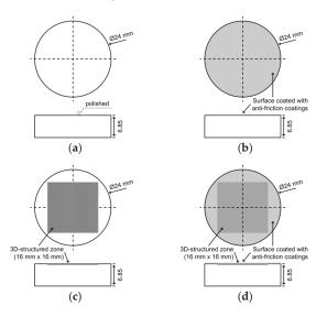
**Figure 2.** Different processed disc surfaces investigated in the present study: (a) benchmark disc, (b) benchmark disc with an antifriction-coating, (c) 3D microtextured disc and (d) 3D microtextured disc with an antifriction coating.
