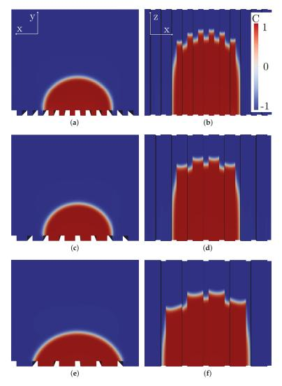
**Figure 3.** Simulation of oil in channels of different widths at t = 0.039 s. The left column (**a**,**c**,**e**) illustrates a cut through the domain at the geometrical center of the droplet. The right column (**b**,**d**,**f**) shows one half of the spreaded droplet filling the channels from the bottom.
