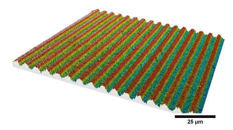
**Figure 6.** Side view of channels from texture S1. This microscopic image demonstrates in an exemplary manner the integrity of the laser produced textures. It can be seen that there are no discontinuities which lead to open structures.
