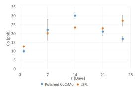
**Figure 7.** ICP-AES analysis of cobalt ion release of polished and LSFL textured CoCrMo samples in ppb as a function of time.
