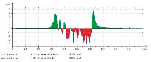
**Figure 3.** Line profile of one of the wear track after a tribo-test, by way of example. The red area represents the worn materials, while the green one is the pile-up.
