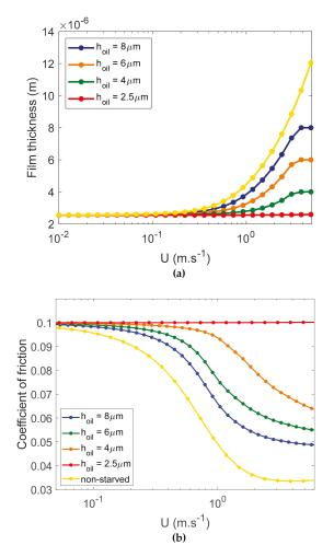
Figure 17. Effect of input film thickness on (a) film thickness, (b) coefficient of friction.
