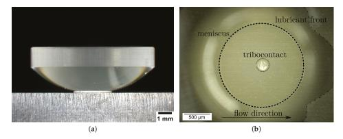
**Figure 10.** In order to elucidate the flow behavior in the transition region between channels and tribocontact a transparent glass lense made of N-BK7 is used as a substitute for the counterbody. (a) A side view of the glass lens on top of a textured sample; in (b) the lens is manually put into the tribocontact and the flow around the lens is observed through the lens with a microscope.
