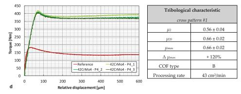
**Figure 13.** SEM micrographs showing the cross pattern made with 2 scan passes (**a**) before and (**b**) after friction testing and (**c**) the counter body surface after the friction test; the recorded slipping curves (**d**) and a summary of the tribological characteristic of the cross pattern texture are presented (table bottom, right).
