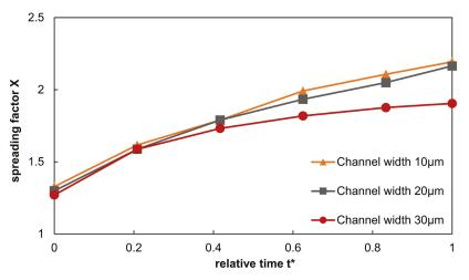
**Figure 4.** Quantitative evaluation of the numerical results comparing the spreading factor  $\chi$  for the different channels widths as a function of the relative time  $t^*$ .
