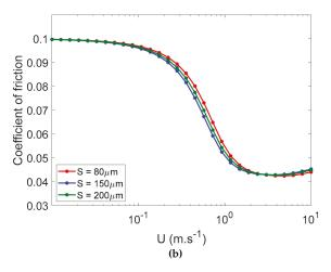
**Figure 14.** Stribeck curves as a function of cavity size for chevrons when the lubrication is: (a) Non-starved, (b) starved, and  $h_{oil} = 10 \mu m$ .
