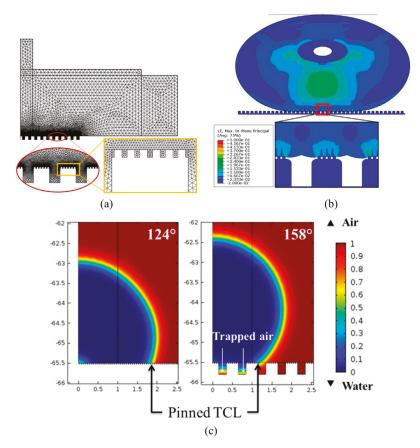
Figure 12. Hierarchical textured surface for anti-fingerprint and self-cleaning applications. (a) Finite element mesh. (b) Deformed shape and strain distribution. (c) Contact angle and wetting state for hydrophobicity analysis. Adapted from [102].
