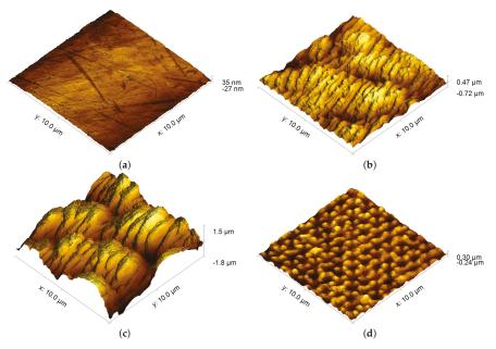
**Figure 5.** AFM micrographs of a CrCoMo surface: unprocessed (**a**), LSFL (**b**), grooves with superimposed LSFL (**c**) and triangular nanopillars (**d**). (**a**) AFM micrograph of polished CrCoMo sample. (**b**) AFM micrograph of LSFL. (**c**) AFM micrograph of Grooves + LSFL. (**d**) AFM micrograph of Triangular Nanopillars.
