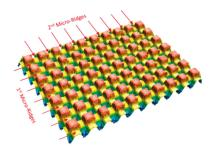
Figure 3. Example of the desired 3D surface microtexture to be produced using an ultra-short pulsed laser on one side of disc specimens.
