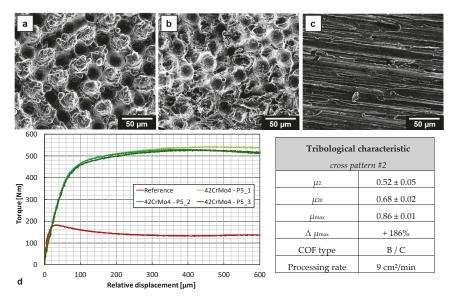
**Figure 14.** SEM micrographs showing the cross pattern made with 10 scan passes (**a**) before and (**b**) after friction testing and (**c**) the counter body surface after the friction test; the recorded slipping curves (**d**) and a summary of the tribological characteristic of the cross pattern texture are presented (table bottom, right).
