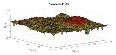
**Figure A3.** Surface roughness profile based on the Laser Scanning Microscope measurements  $(R_a = 0.11 \, \mu \text{m})$ .
