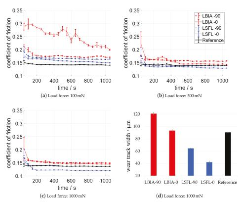
**Figure 6.** Tribological evaluation using 100Cr6 triboballs under lubrication. Temporal evolvement of the coefficient for a load force of 100 mN (**a**), 500 mN (**b**), and 1000 mN (**c**). Wear track width on the 100Cr6 substrate after after 1000 s test duration using a load force of 1000 mN and 100Cr6 triboballs (**d**).
