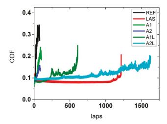
Figure 8. COF versus laps in order to determine the maximum oil film lifetime of the polished reference, the cross-like laser textures (LAS), the micro-coined surfaces (A series) and both corresponding multi-scale textures (A1L and A2L). Adapted from [70].
