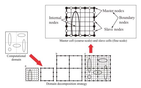
**Figure 17.** Overview of the finite cell method proposed by [227] for modeling surface textures in different lubrication regimes. (a) Illustration of the main domain decomposition steps and nomenclature of the proposed method.
