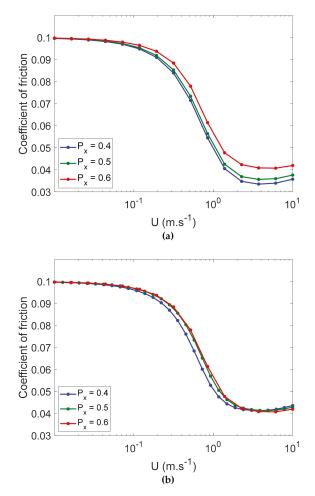
**Figure 15.** Stribeck curves as a function of texture pitch for grooves when the lubrication is: (a) Non-starved, (b) starved, and  $h_{oil} = 10 \,\mu\text{m}$ .
