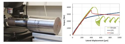
**Figure 15. left:** Topographical analysis of the shaft, the laser textured area is on the left shaft end; **right**: slipping curves captured in the frictional tests using a test rig for joined real components.
