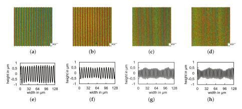
Figure 5. Microscope pictures and profiles of laser textures evaluated in this study. Textures and profiles of S1 (a) and (e), S2 (b) and (f), S3 (c) and (g) and S4 (d) and (h).
