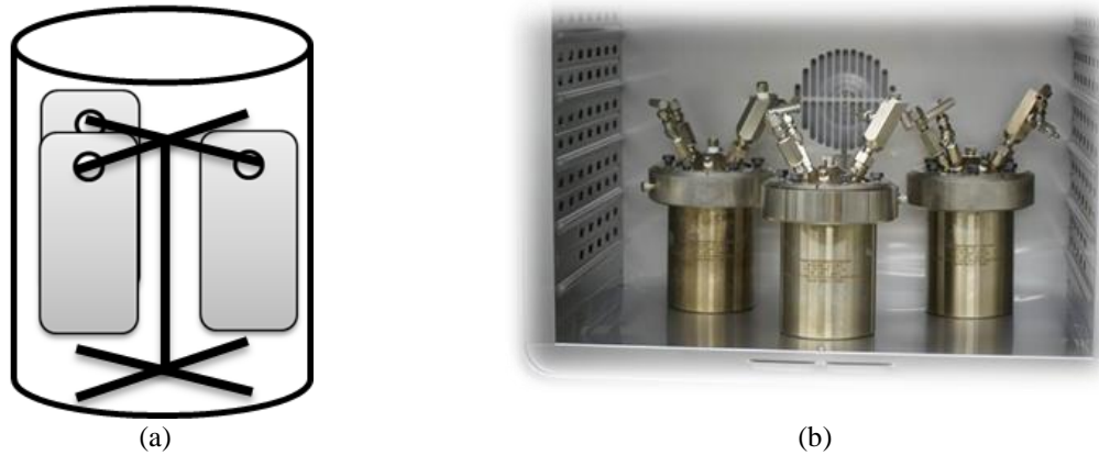
Figure 3.10. Exposure test set-up for higher temperatures: (a) illustration of specimen arrangement inside the autoclave, and (b) image of autoclaves
