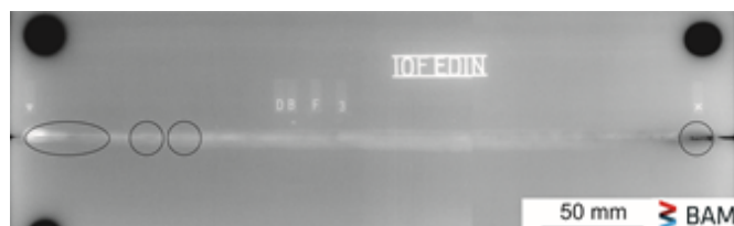
Fig. 7. X-ray image of a single-pass weld seam with defects (black circled)
