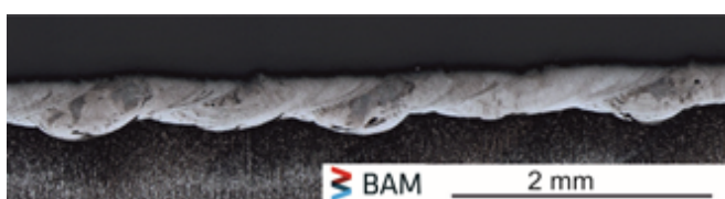
Fig. 4 Cross section of buttered edge
